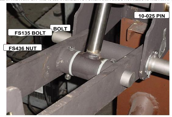
REMOVE THE 4ea FS442 3/4-10 NYLOCK NUTS AND THE FS334 3/4 INCH FLAT WASHERS FROM THE 10-010 PINS. THERE IS A N AND WASHER ON BOTH ENDS OF THIS PIN. DO NOT RE MOVE PIN AT THIS TIME.
