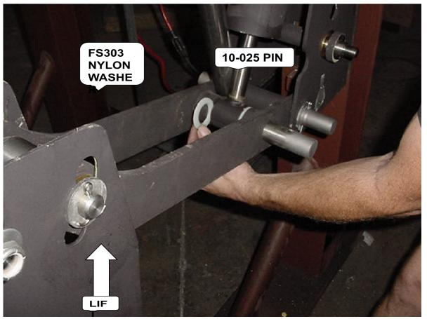
SUPPORT THE 10-039 3" BRAVO CYLINDER TO PROTECT THE ROD WITH THE PLATFORM BRACKET RESTING ON THE GROUND,
