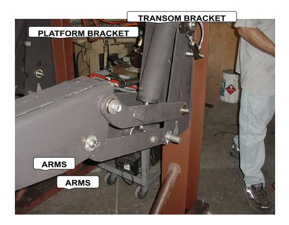
REMOVE THE 2 ea 1/4-20x2 1/2 INCH BOLTS AND NUTS CLEAN THE PAINT OFF THE 10-025 CYLINDER TO POWER ARM PIN. DO NOT REMOVE THE PIN AT THIS TIME.
