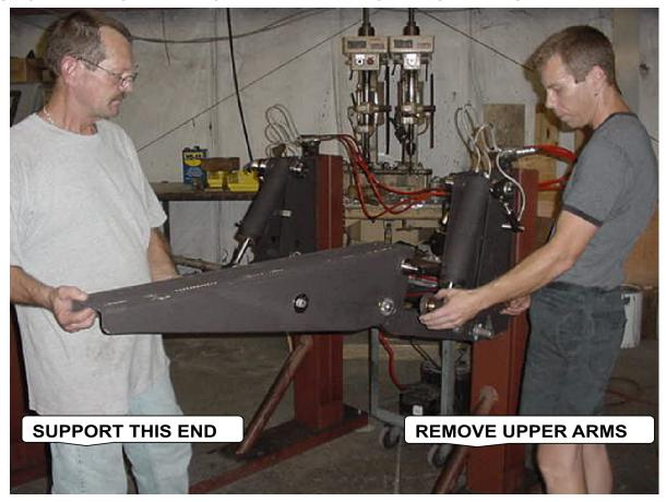
WITH BOTH UPPER ARMS REMOVED, ROTATE THE PLATFORM BRACKET DOWN.
