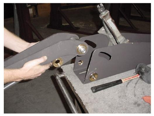
10-003 BRASS BUSHINGS ARE 1.25" ID AND 1.5" OD QTY 12 PER LIFT 10-021 BRASS BUSHINGS ARE 1" ID AND 1.5" OD QTY 20 PER LIFT
